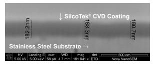
SilcoTek® CVD coatings are thin flexible barriers that increase the lifetime of critical components in corrosive environments. The coatings are typically 500-1500nm thick.
