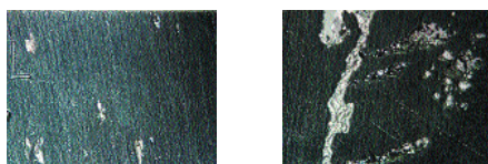
Figure 2 Silcolloy 1000 treated 316L stainless steel coupons show no crevice corrosion and only slight pitting corrosion after 72-hour exposure to ferric chloride; untreated coupons exhibit severe crevice corrosion (per ASTM Method G48, Method B).
