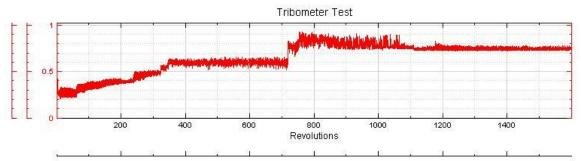
Figure 4: Graph of COF for Oxidized Steel
