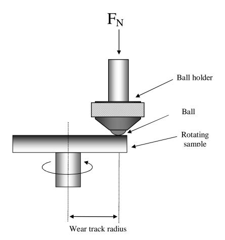
Figure 3 : Schematic of the contact on the sample
