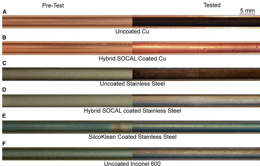
**Figure 1. Optical images of the cross-sectioned tube samples before and after the fuel fouling experiment**
