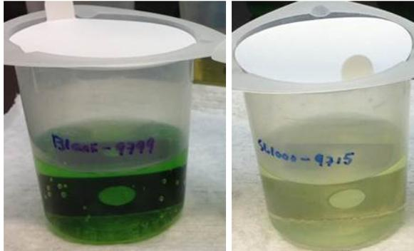
$$\text{Corrosion Rate} = \frac{\text{Weight loss (g)} \cdot \text{K-factor}}{\text{Density (g/cm}^3\text{)} \cdot \text{Area (A)} \cdot \text{Time (hr)}}$$
