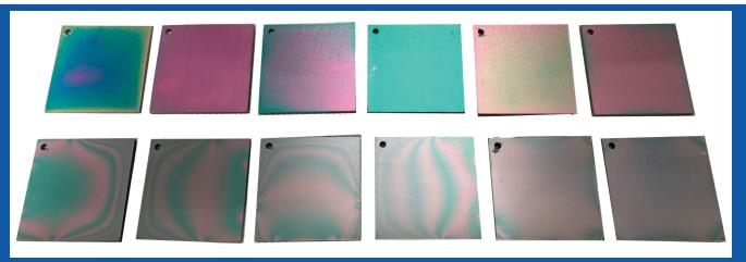
SilcoNert's light refraction properties above correlate with a coating thickness between 100 to 500 nm (from right to left: thin to thick). The light spectrum produced by the SilcoNert coating process is more vibrant than Dursan and includes deep blues, purple, green, and gray. The coupons shown above are highly polished, resulting in a bright color spectrum. Rough and unpolished steel surfaces will subdue the colors.
