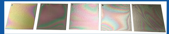
Dursan's light refraction properties (seen above) correlate with a coating thickness between 400 and 1600 nm. The refraction properties of the Dursan coating process are more subtle than SilcoNert, making it easy to distinguish between the two.
