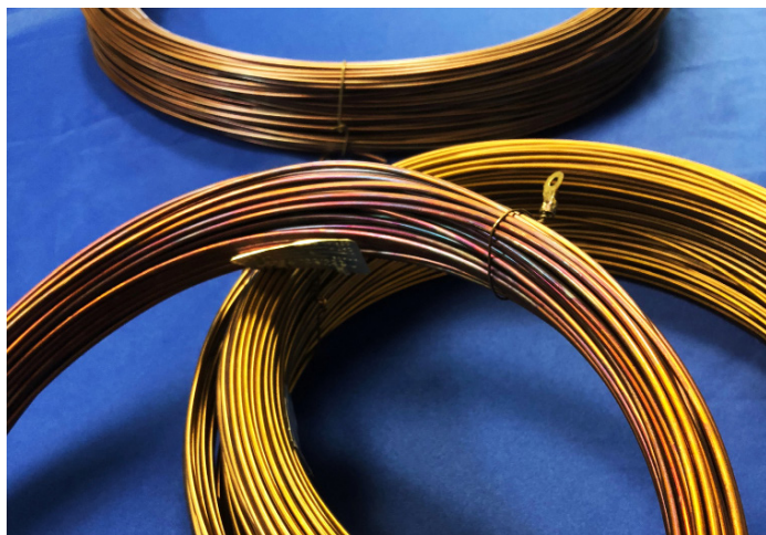
The exterior of coated tubing can vary from yellow to golden brown to even purple due to metal oxidation in air.
