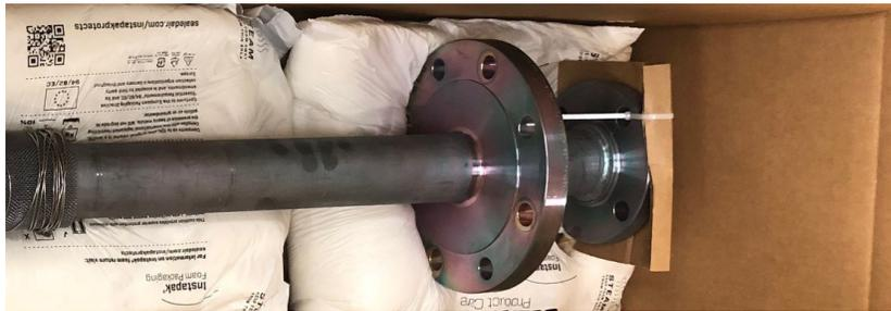
Image 1 (above) depicts a sampling probe where the customer was concerned about inaccurate measurement of sulfides in the collected samples. It was believed that the skewed measurements originated from cross-contamination of sulfide leaching into the metallic sample cylinder and system components. A SilcoNert 2000 coating was applied to the probe, providing an inert and corrosion resistant barrier that will prevent any metal ion leaching or contamination of the sulfide readings.
