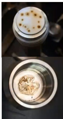
Figure 4: Corrosion on customer parts.
