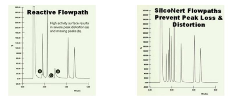
An inert flowpath will prevent signal loss, improve response and improve peak quality; making calibration faster and easier.
