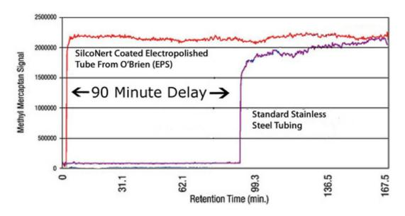
Adsorption will delay or even prevent accurate testing. Reactive surfaces like stainless steel can significantly impact results, so an inert flow path is a critical feature in the sampling system for maximum reliability.
