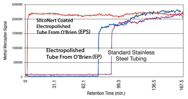
Analyzing highly active sulfur compounds like methyl mercaptan (CH<sub>3</sub>SH) once required "priming" or "seasoning" of the system to get an accurate signal, adding hours to overall analysis times. Today, inert-coated sample flow paths allow for instant and accurate readings of these reactive analytes (red line above).
