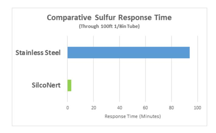
Active sites in the uncoated tube grab onto the sulfur sample, preventing it from reaching the analyzer for 90 minutes! Excessive delay in signal response will make process control almost impossible.
