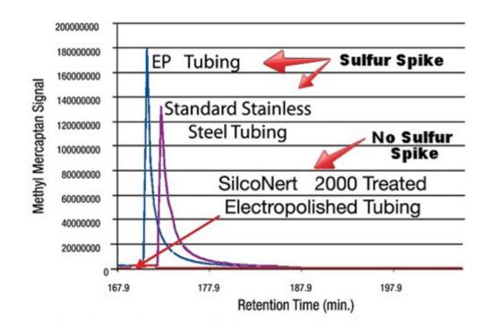
Desorption or delayed release of compound from a reactive surface can lead to false or misleading results.
