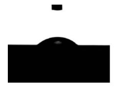
Low energy surfaces that don't wet and produce a high contact angle may be less reactive to your analyte.
