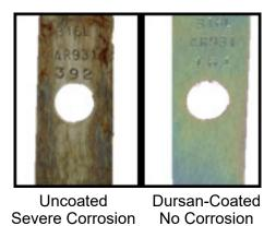
EIS (<u>Electrochemical Impedance Spectroscopy</u>) data show Dursan remains pinhole free after over 250 days of salt spray exposure. In the experiment below, test coupons are subjected to salt spray for 247 days. The test samples were periodically tested by introducing a voltage between 5 to 50 mV with a range of frequencies. If the resulting data points do not diverge or curve, no additional pin holes were produced.
