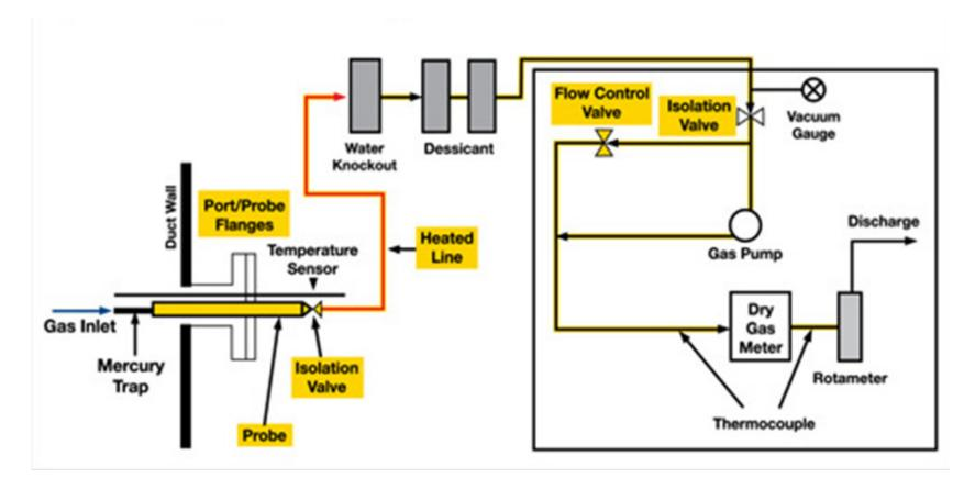
Typical stack sampling train. SilcoTek<sup>®</sup>-coated flow paths will prevent adsorption of mercury, ammonia, and sulfur compounds, assuring reliable compliance monitoring.
