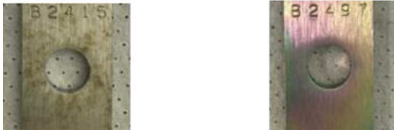
Figure 1: A bare stainless steel coupon (left) and a Dursan coated stainless steel coupon (right) were exposed to guanidine hydrochloride for one month. The rusting on the bare coupon is more severe than the 1 week exposure. As seen previously, the Dursan coated coupon is unaffected by the exposure.
