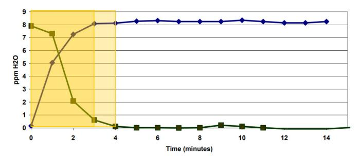
Moisture Analyzer Response on Wetup / Drydown
