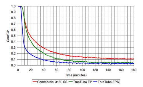
Desorption testing provided similar relative performance improvements for TrueTube<sup>™</sup> EP and TrueTube<sup>™</sup> EPS over commercial seamless sample transport tube. Equivalent reductions in moisture were reached in 35 minutes for TrueTube<sup>™</sup> EPS and 65 minutes for TrueTube<sup>™</sup> EP while commercial seamless tubing took 175 minutes.
