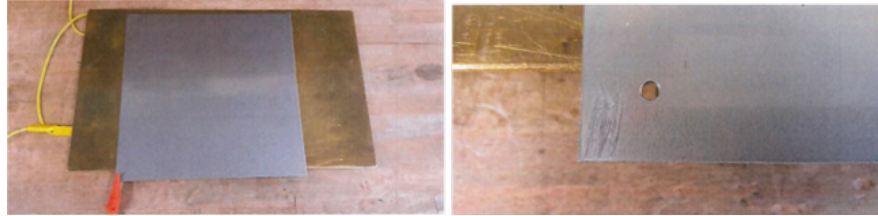
Figure 1: Electrostatic safety test setup showing the Dursan-coated plate and the scraped corner for ground clamp connection
