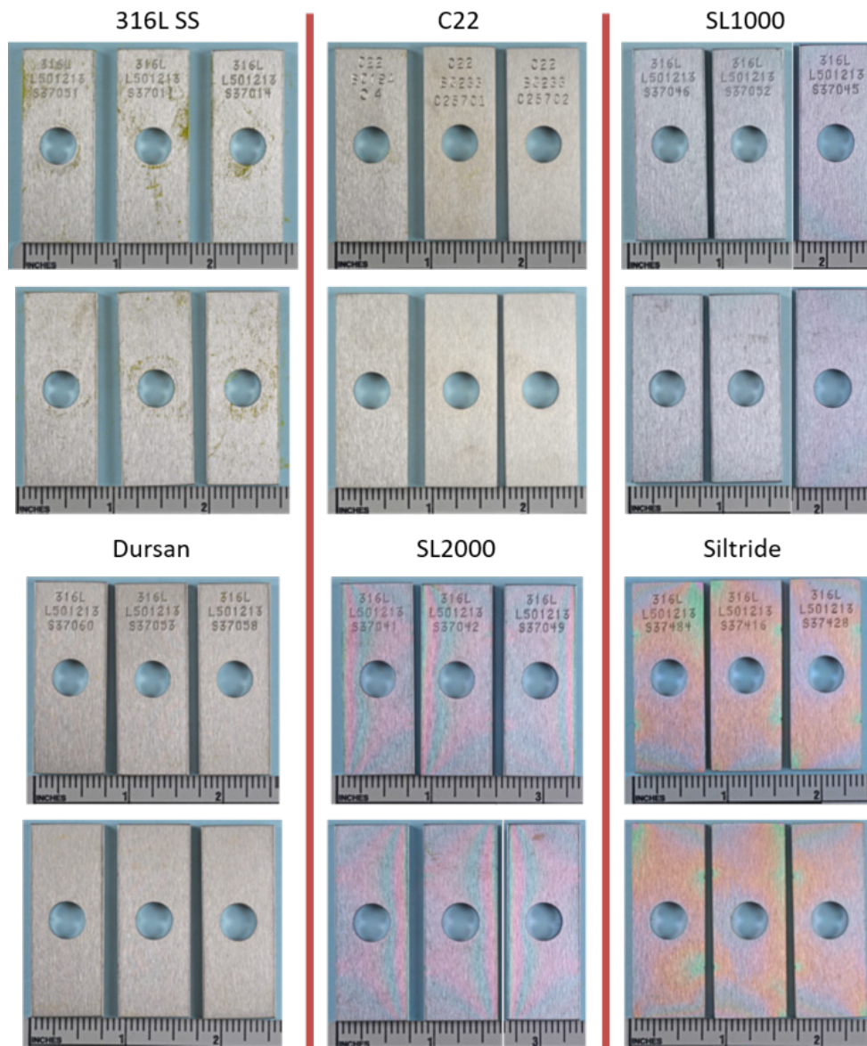
Figure 2: Photographs of all coupons (front and back side) immediately after removal from the room temperature test vessel without any rinsing
