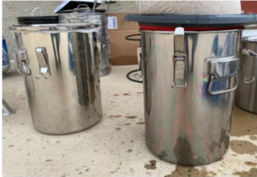
Figure 3: Chapman all-in-one brewing systems. On the left is the uncoated example and the right is the Dursan coated system.
