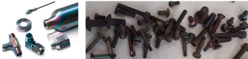
Figure 1: typical SN2000 output on SS parts (left), and SN2000 coating on a batch of customer-supplied silver-plated SS screws (right)
