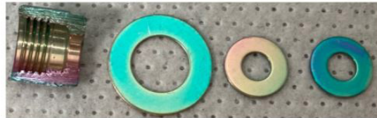
Figure 3: SN2000-coated Swagelok compression nut and VCR gaskets appear normal (all silver-plated)
