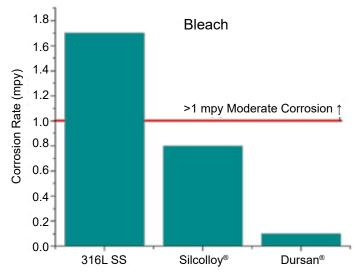
SilcoTek® coatings (right) allow the use of concentrated bleach without any of the corrosion issues that are common with bare stainless steel.
