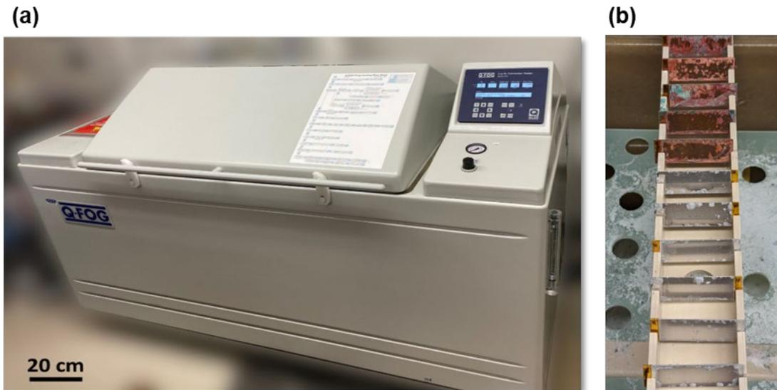
Figure 4: (a) Q-fog cyclic corrosion chamber. (b) Arrangement of samples inside the testing chamber
