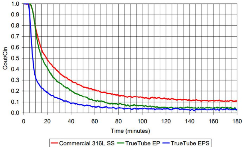
Desorption testing provided similar relative performance improvements for TrueTube™ EP and TrueTube™ EPS over commercial seamless sample transport tube. Equivalent reductions in moisture were reached in 35 minutes for TrueTube™ EPS and 65 minutes for TrueTube™ EP while commercial seamless tubing took 175 minutes.
