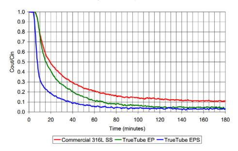
Desorption testing provided similar relative performance improvements for TrueTube™ EP and TrueTube™ EPS over commercial seamless sample transport tube. Equivalent reductions in moisture were reached in 35 minutes for TrueTube™ EPS and 65 minutes for TrueTube™ EP while commercial seamless tubing took 175 minutes.
