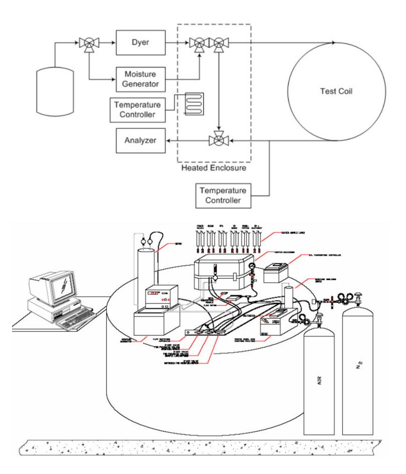
The carrier gas was high purity dry nitrogen. For dry down tests the stream was diverted through a molecular sieve dryer to insure a moisture content of less than 10 ppb.
