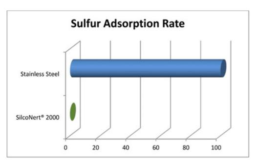
The adsorption caused a significant delay in results but did not account for all the loss.<sup>3</sup> The paper "<u>Do's and Don'ts in the</u> <u>Analysis of Sulfur</u>" by Biela<sup>1</sup> and Reese<sup>2</sup> confirmed refinery's suspicions. The hot stainless steel in the heat trace tubing was causing decomposition of the  $H_2S$ .
