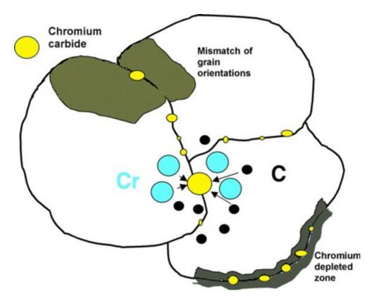
When heated above 500 °C, carbon in the metal grain boundaries of stainless steel will migrate (precipitate) out of the metal to the surface. The overall result is increased susceptibility to corrosion, known as heat sensitization.\*
