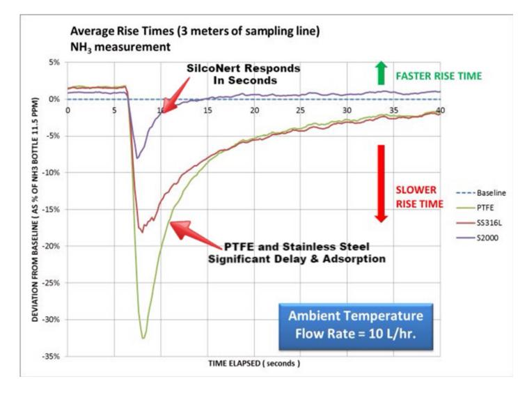
In fact, test errors can be significant; initial NH<sub>3</sub> signal rise time results show major differences:
