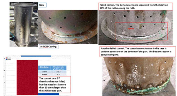
Figure 10. Photographic images of a new control Part B at the top-left of the graphic. Next, a Part B coated with SiON shows little corrosion. A failed, control Part B is shown at the top-right of the graphic. The failure mechanism is SCC (Stress Chemical Corrosion). By contrast, the failure mechanism of the control Part B shown at the bottom-right is bulk corrosion. The bar chart at the bottom-left shows the etch rate of the control is about two orders of magnitude higher than the control.
