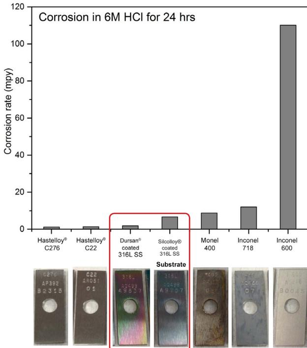
SilcoTek® CVD coatings offer the corrosion performance of super alloys at a fraction of the cost when applied to stainless steel.
