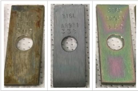
SilcoTek®-coated 316L stainless steel (middle, right) is completely unaffected by ASTM G85-A2 salt spray testing after 8000+ hours.
