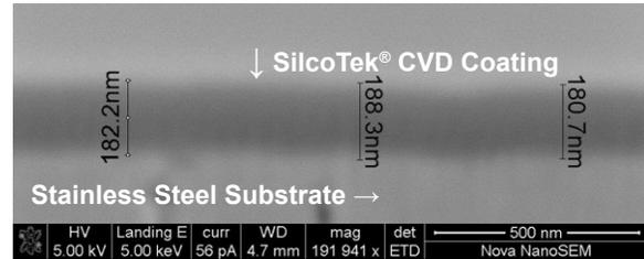
SilcoTek® CVD coatings are thin flexible barriers that increase the lifetime of critical components in corrosive environments. The coatings are typically 500-1500nm thick.
