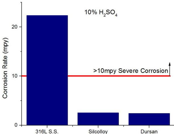
Even in aggressive sulfuric acid conditions, SilcoTek® CVD coatings provide stable protection for higher system output.
