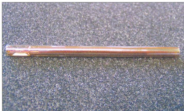
Figure 1: Sintered glass insert with glass beads on inner surface for Optic 3 with SILTEK deactivation
