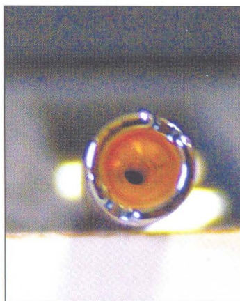
Figure 1: Sintered glass insert with glass beads on inner surface for Optic 3 with SILTEK deactivation
