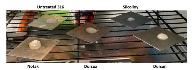
Upon opening the freezer door (see photo), each coupon was individually removed and rapidly tested to avoid the potential impact of thawing. A metal pick inserted at the point of ice attachment to the coupon was used to laterally remove the ice. The effort required (1 = easy, 10 = difficult) to remove the ice and associated observations are listed in the table below.
